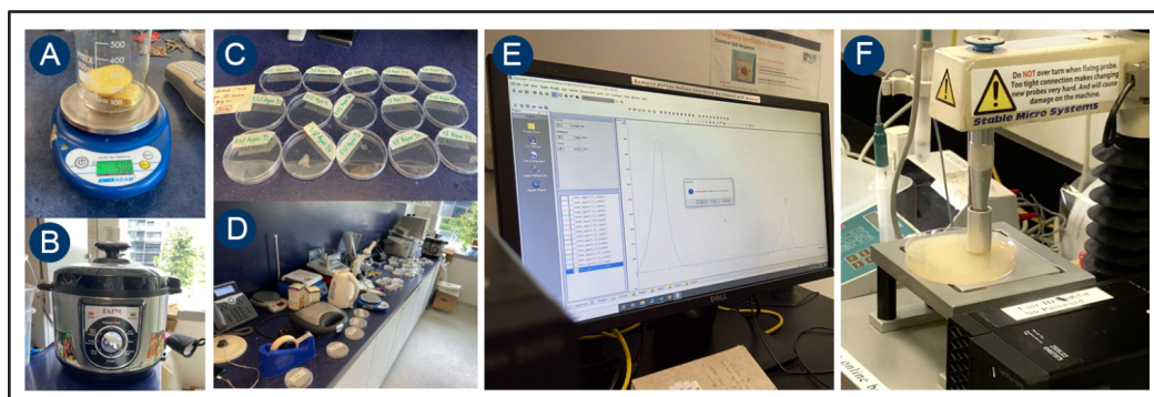
Fig. 2 A-D. The process of making potato dextrose agar(PDA) media for yeast cultivation. E-F. Using Texture Analysis Profile to collect data of mechanical forces, hardness and resilience.
